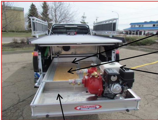
SMARTBOX houses the pump tray.
